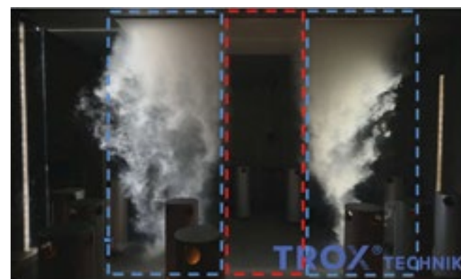
The design of the TFM ceiling tile minimises air mixing between temperature zones.
