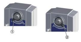
Fig. 222: Damper blade position indicator
