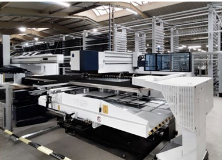
Laser punching machine in sheet metal pre-production at the Anholt production facility
